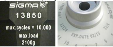
Fig. 5.9: Different service life – engraving on the bucket/rotor
