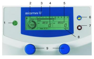
Fig. 5.4: Operating panel with centrifuge display
