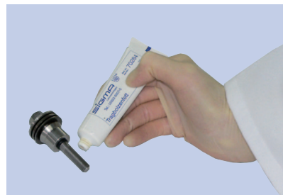
Fig. 4: Greasing the rotor tie-down screw
