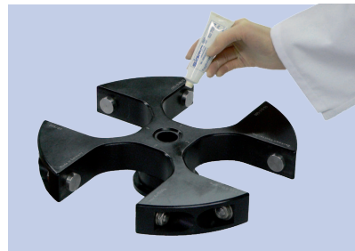
Fig. 2: Greasing the load-bearing bolts (very thin layer)
