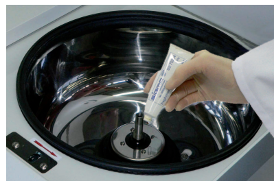
Fig. 3: Greasing the motor shaft (very thin layer)
