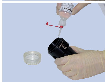
Fig. 6: Applying slushing oil to the lid seal of a bucket
