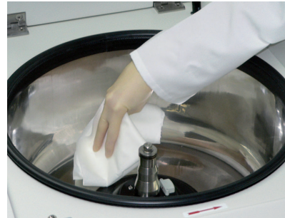
Fig. 1: Cleaning the rotor chamber
