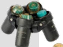
A black, angled rotor with 4 slots for 100 ml tubes. The lid is shown slightly offset from the base.
