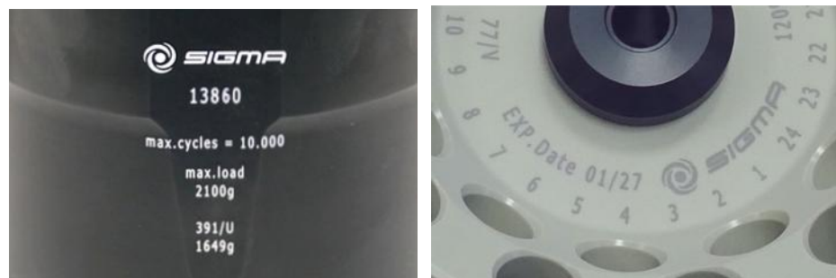
Fig. 8: Different service life – engraving on the bucket/rotor
