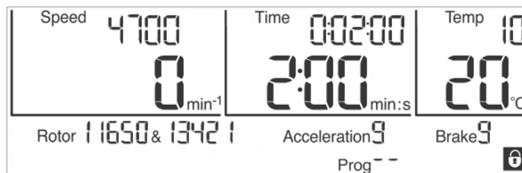
Fig. 32: "Padlock" symbol indicating an activated input lock
