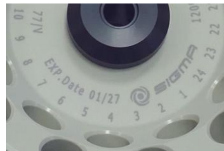
Fig. 7: Different service life – engraving on the bucket/rotor
