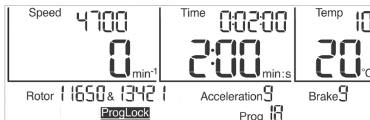
Fig. 29: The program lock "ProgLock" is activated
