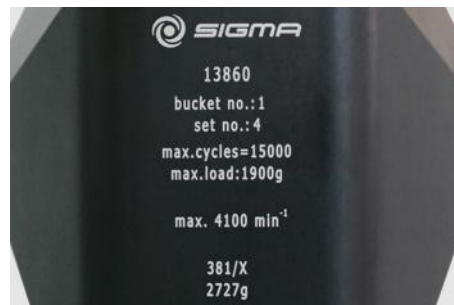
Fig. 7: Different service life – engraving on the bucket/rotor
