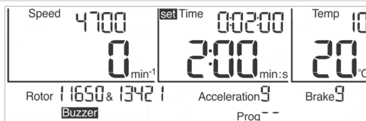
Fig. 19: Setting the runtime, here in the time unit "min:s"
