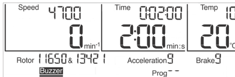
Fig. 28: The sound signal "Buzzer" is activated
