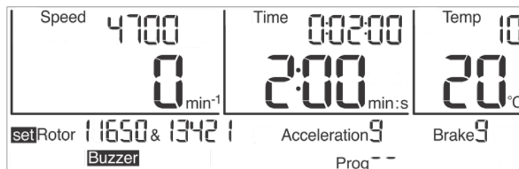
Fig. 25: Preselection of a rotor or a rotor/bucket combination
