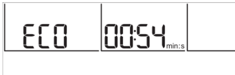
Fig. 33: Indication of the last 29 minutes of the countdown before the activation of the Eco mode
