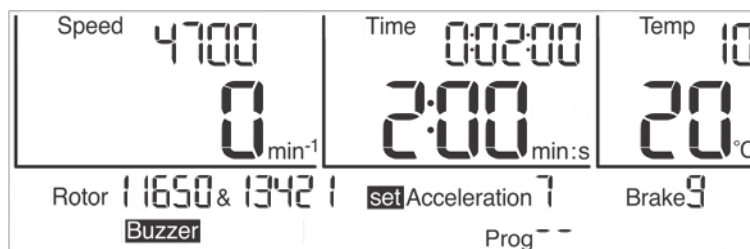
Fig. 26: Preselection of a curve; here: preselection of an acceleration curve
