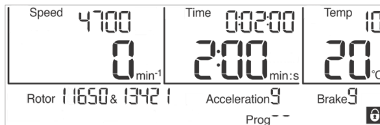
Fig. 31: "Padlock" symbol indicating an activated input lock
