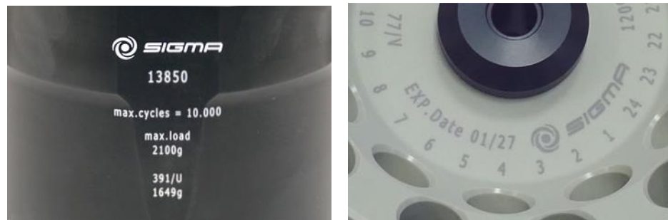
Fig. 6: Different service life – engraving on the bucket/rotor
