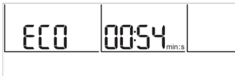
Fig. 32: Indication of the last 29 minutes of the countdown before the activation of the Eco mode
