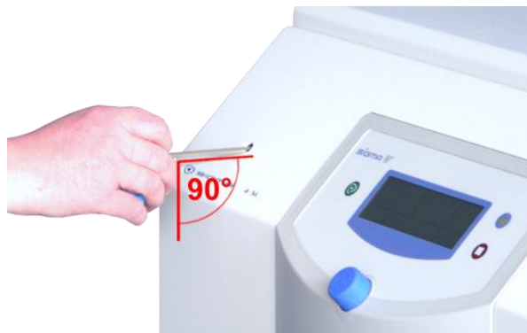
Fig. 38: The emergency lid release key must be inserted horizontally (example illustration)
