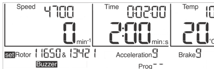
Fig. 24: Preselection of a rotor or a rotor/bucket combination
