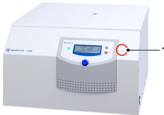
Fig. 37: Position of the opening for the emergency lid release
