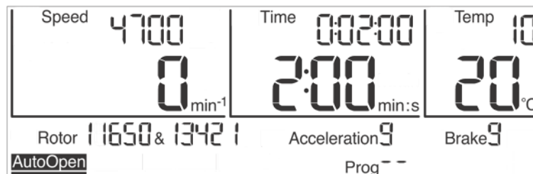
Fig. 26: The automatic lid opening function "Auto Open" is activated
