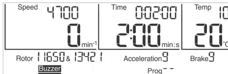
Fig. 27: The sound signal "Buzzer" is activated
