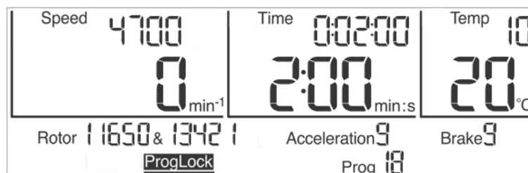
Fig. 28: The program lock "ProgLock" is activated
