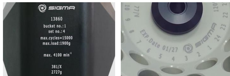
Fig. 5: Different service life – engraving on the bucket/rotor
