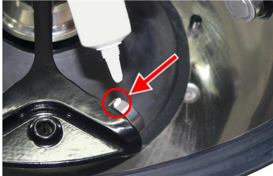
Fig. 37: Sufficient quantity of grease for one bolt
