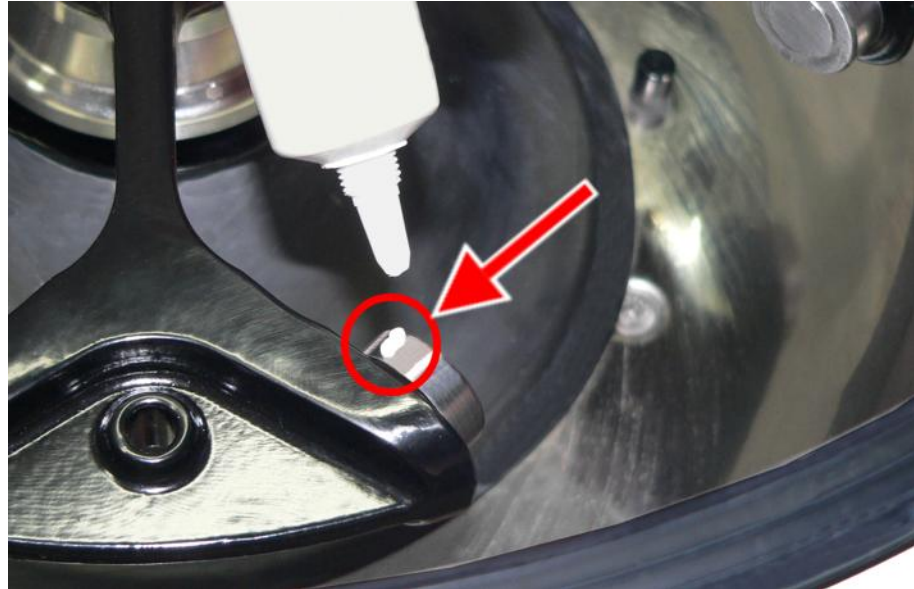
Fig. 36: Sufficient quantity of grease for one bolt
