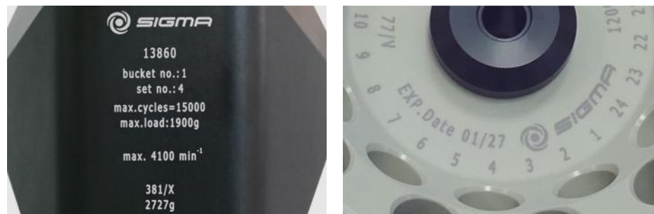
Fig. 5: Different service life – engraving on the bucket/rotor
