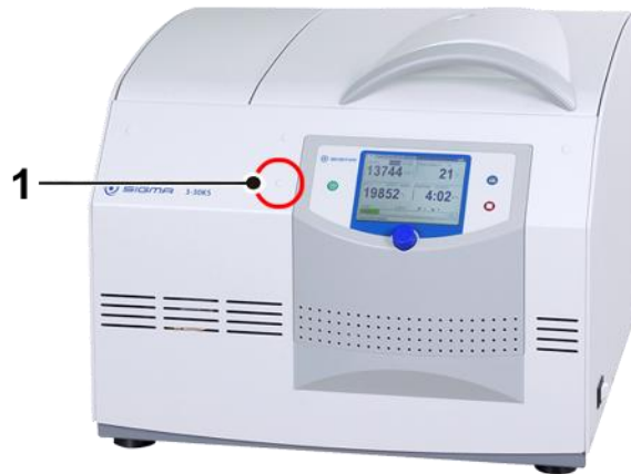
Fig. 34: Position of the opening for the emergency lid release
