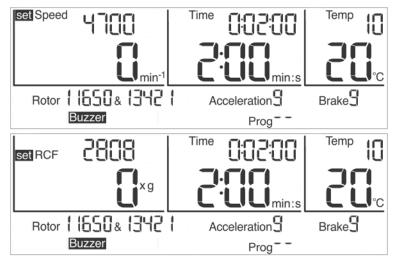
Fig. 16: Setting the speed value or the RCF value
