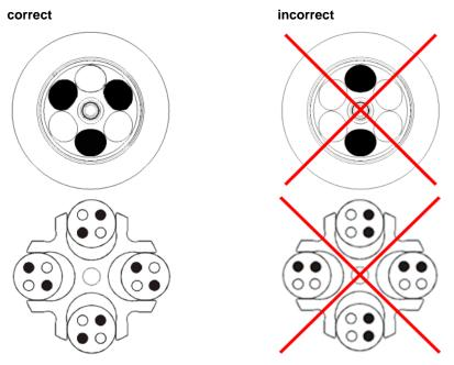
Fig. 12: Permissible and impermissible loading of an angle rotor and a swing-out rotor (example illustrations)
