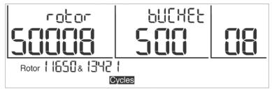
Fig. 29: Display when the maximum number of cycles is reached (flashing)
