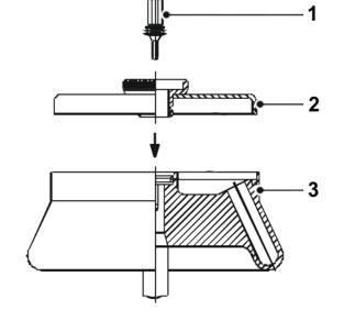
Fig. 10: Angle rotor with a hermetic lid
