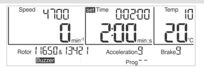
Fig. 17: Setting the runtime, here in the time unit "min:s"
