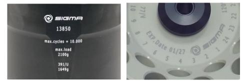
Fig. 4: Different service life – engraving on the bucket/rotor
