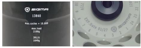
Fig. 5: Different service life - engraving on the bucket/rotor
