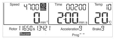
Fig. 18: The function "Runtime as of the set speed" is activated
