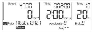
Fig. 23: Preselection of a rotor or a rotor/bucket combination
