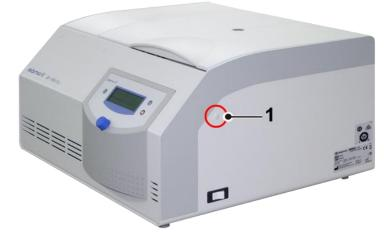
Fig. 33: Position of the opening for the emergency lid release
