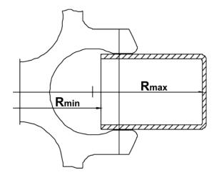
Fig. 36: Minimum and maximum radius of a swing-out rotor
