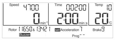
Fig. 24: Preselection of a curve; here: preselection of an acceleration curve
