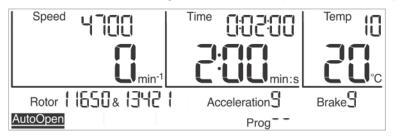
Fig. 25: The automatic lid opening function "Auto Open" is activated
