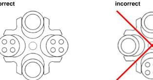
Fig. 11: Permissible and impermissible loading of a swing-out rotor with vessels of various sizes (example illustration)
