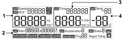
Fig. 15: Display of the Spincontrol L control system
