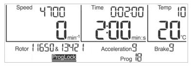
Fig. 27: The program lock "ProgLock" is activated
