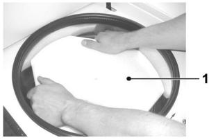
Fig. 9: Removal of the transport safety device (example)
