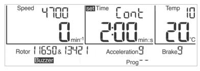
Fig. 19: Indication "Cont" during a continuous run
