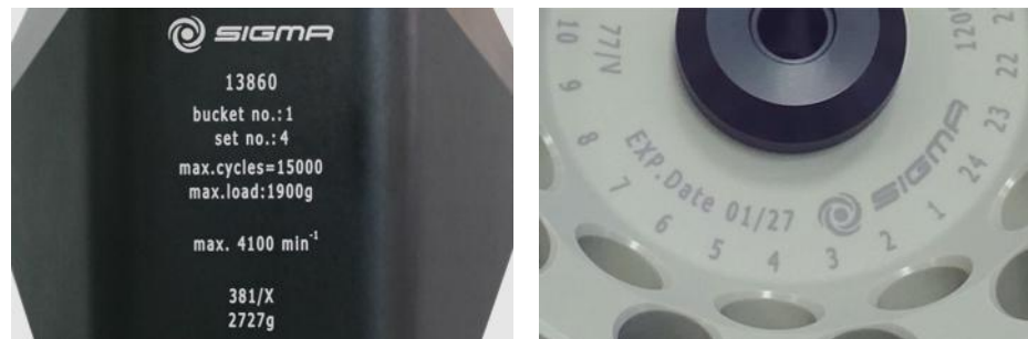
Fig. 4: Different service life – engraving on the bucket/rotor
