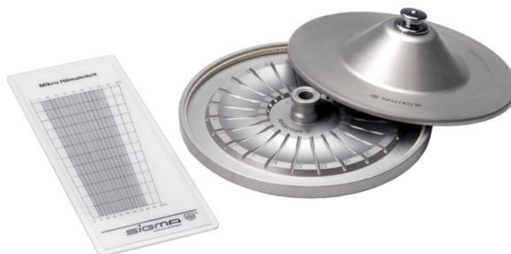
Fig. 5: Microhaematokrit rotor (part no. 11026) with reader (part no. 17028)
