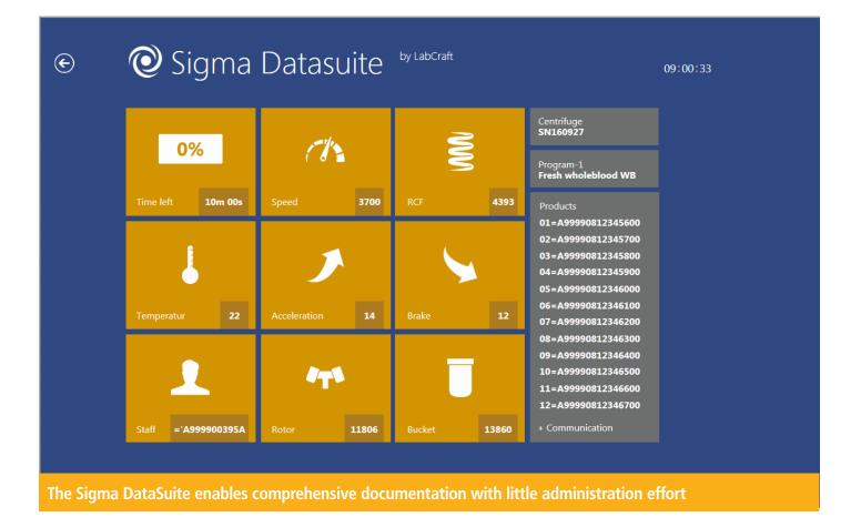
Sigma Datasuite continuously monitors the status of the connected centrifuges and will automatically write a file to a user-defined location once a centrifugation run is completed.
