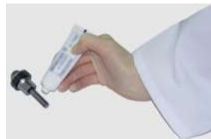
Fig. 4: Greasing the rotor tie-down screw
