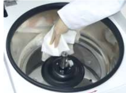
Fig. 1: Cleaning the rotor chamber
