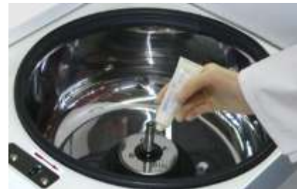
Fig. 3: Greasing the motor shaft (very thin layer)
