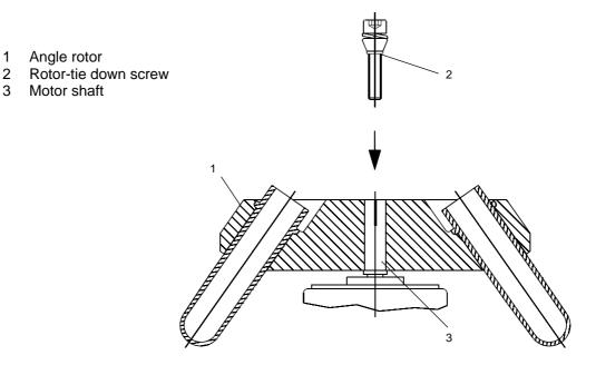
Fig. 5.5: Installation of a rotor
