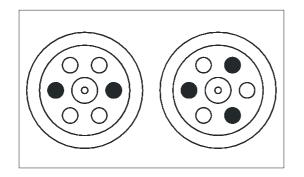
*Fig. 5.6:* Correct loading of the angle rotor
