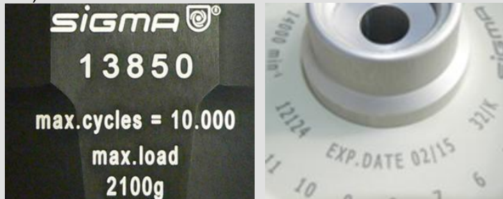
Fig. 3.1: Different service life – engraving on the bucket/rotor
