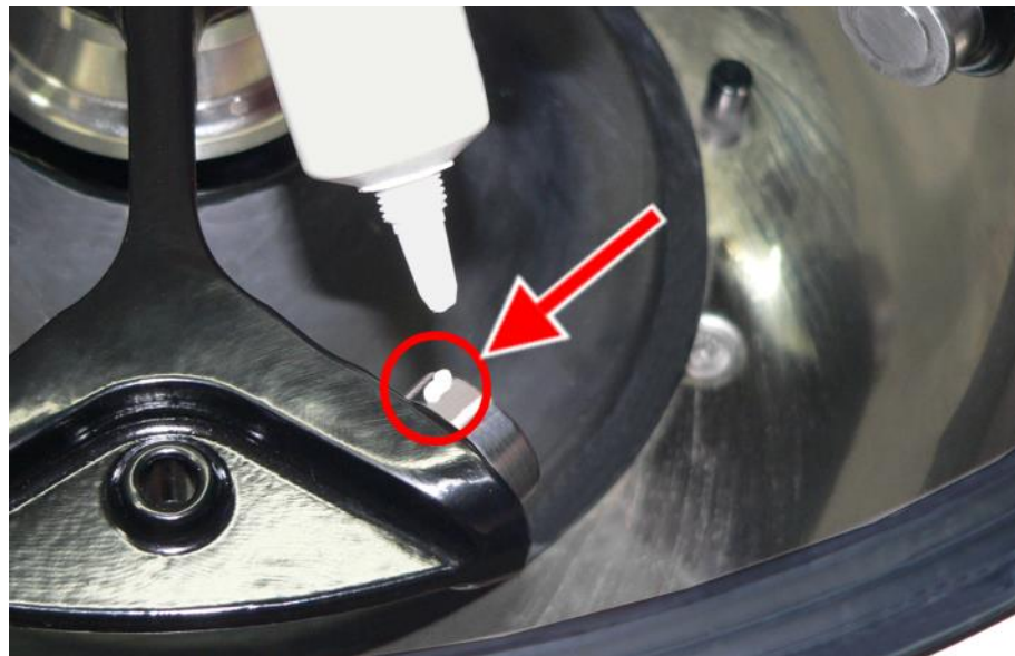
Fig. 25: Sufficient quantity of grease for one bolt
