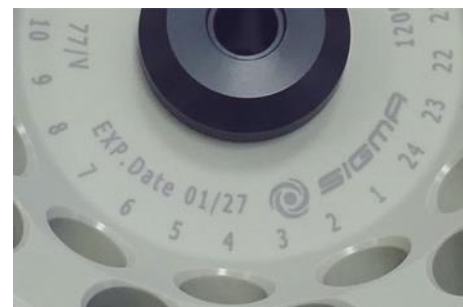
Fig. 4: Different service life – engraving on the bucket/rotor
