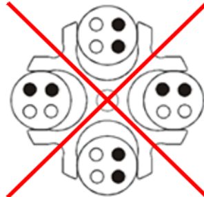
Fig. 10: Permissible and impermissible loading of an angle rotor and a swing-out rotor (example illustrations)
