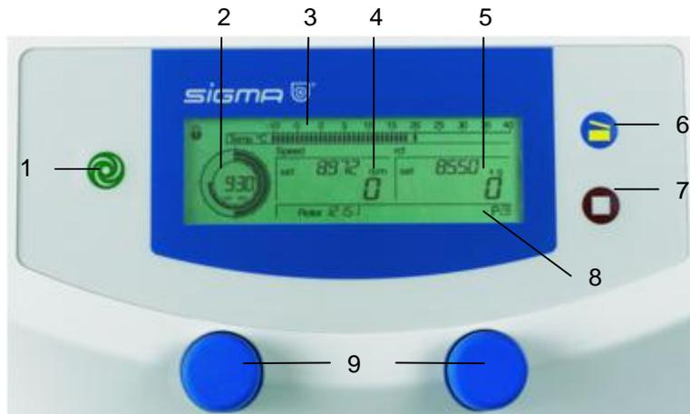
Fig. 5.4: Operating panel with centrifuge display
