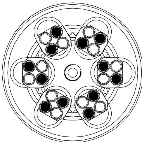
Fig. 5.8: Permitted loading of the swing-out rotor 24 x 2,2 ml
