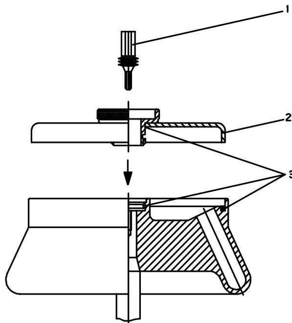
Fig. 5.6: Angle rotor with a hermetically sealed lid
