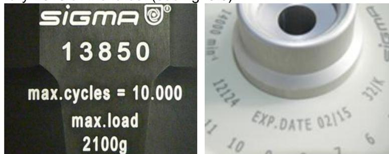
Fig. 5.9: Different service life – engraving on the bucket/rotor
