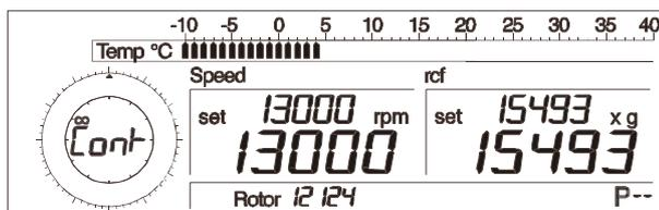
Fig. 5.13: Continuous run display
