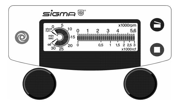
The centrifuge is operated via the operating panel. Keys can be pressed when their LED is on.
