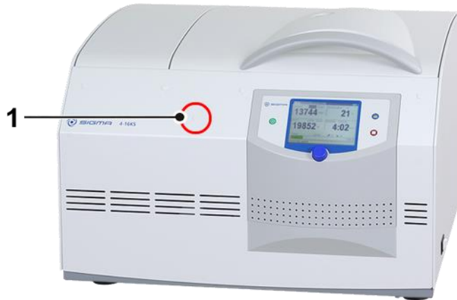
Fig. 34: Position of the opening for the emergency lid release
