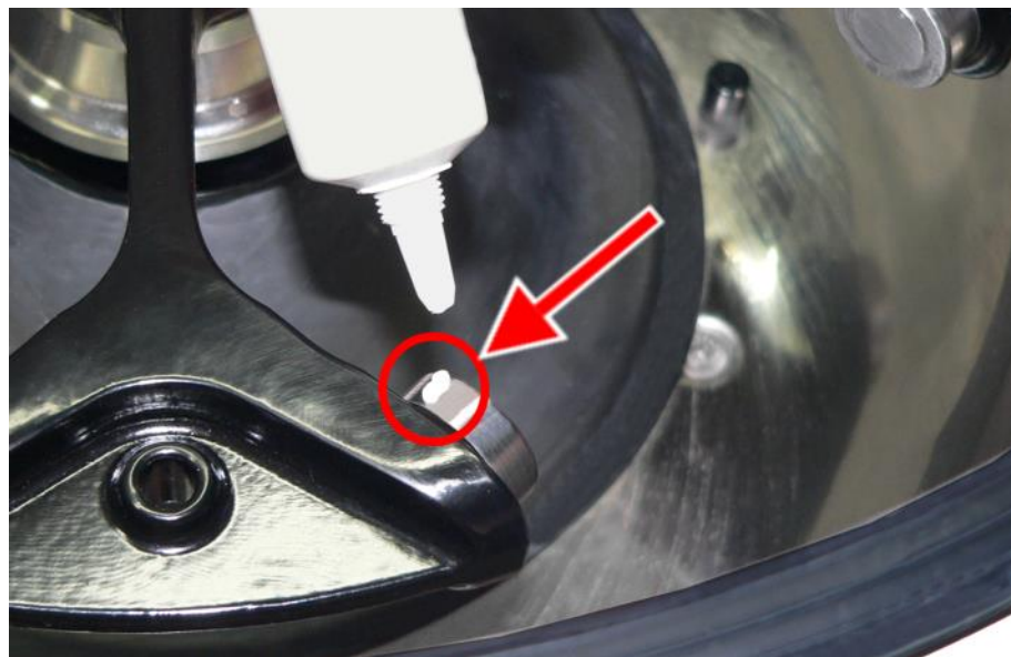
Fig. 36: Sufficient quantity of grease for one bolt
