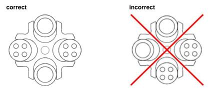
Fig. 10: Permissible and impermissible loading of a swing-out rotor with vessels of various sizes (example illustration)
