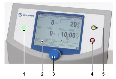
Fig. 13: User interface of the Spincontrol S control system
