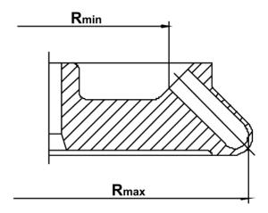
Fig. 35: Minimum and maximum radius of an angle rotor
