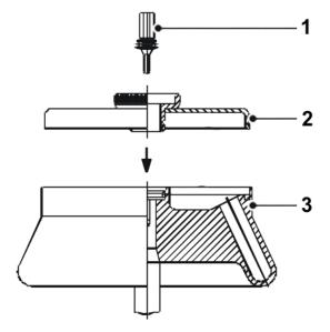
Fig. 9: Angle rotor with a hermetic lid
