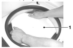
Fig. 8: Removal of the transport safety device (example)
