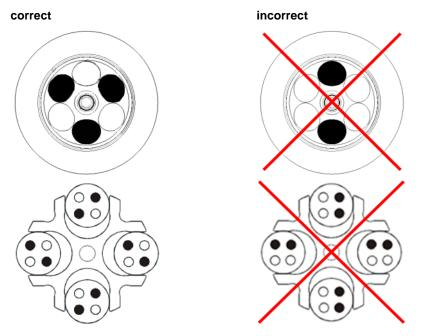
Fig. 11: Permissible and impermissible loading of an angle rotor and a swing-out rotor (example illustrations)
