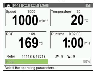
Fig. 19: Progress indicator during a centrifugation run
