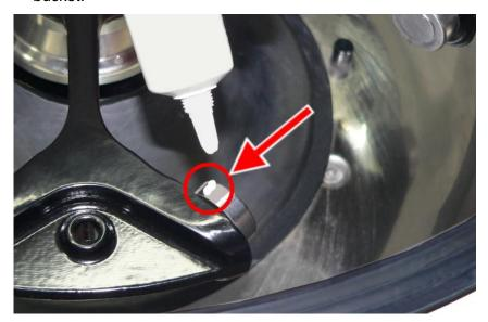
Fig. 34: Sufficient quantity of grease for one bolt
