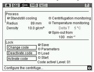
Fig. 23: "Parameters" menu with an active lock (level 01)
