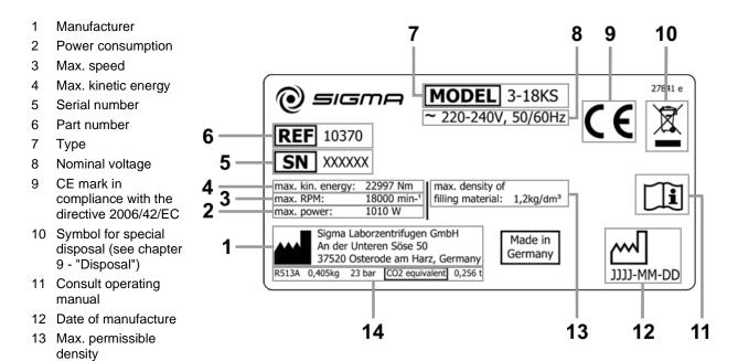
Fig. 3: Example of a name plate
