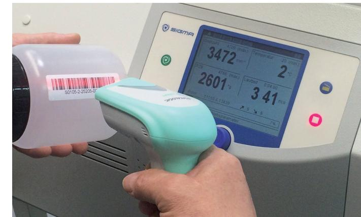
Specimen data is comfortable read via barcode
